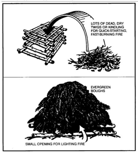
Figure 19-2. Smoke generator-ground.
