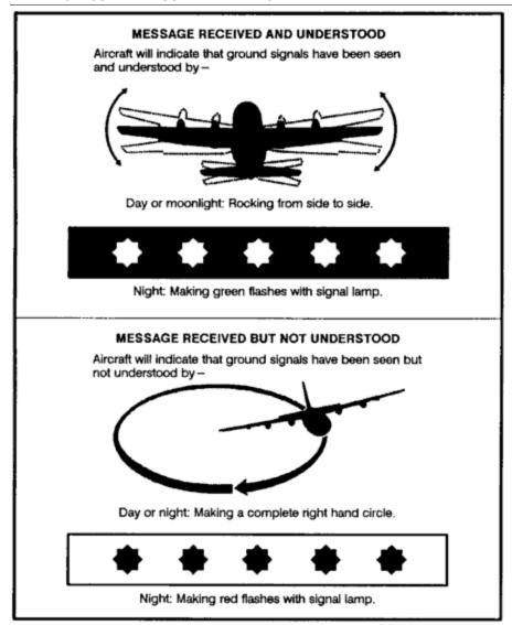
Figure 19-9. Aircraft acknowledgments.
